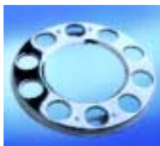
Cover ring, open For aluminium and steel rim 17,5": 1650 1806 steel rim 22,5": 1650 1803 alu rim 22,5": 1650 1804
