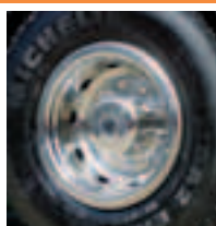
Ornamental hub cap at the rear 22,5" Exklusive, with wheel nut caps, with fixing ring 8060 42075
