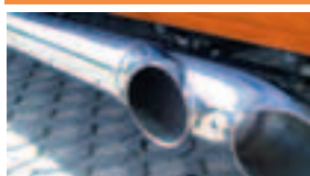
XF/95 XF single outlet No. 1650 5006 dual outlet No. 1650 5015 V4A stainless steel
